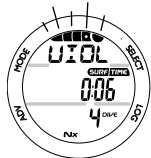
Fig. 88 - VIOLATION GAUGE SURFACE
