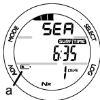
Fig. 3 - LOW BATTERY WARNING
