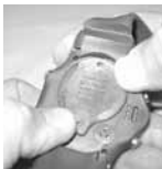
Fig. 123 - BATTERY COVER O-RING (without tool)
